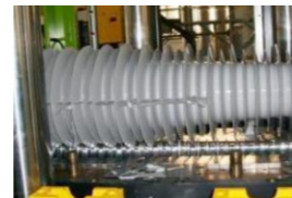
制品名称: 110kV锥形管套 成型腔数: 一出二 Part Name: 110kV Cone Type Hollow Core Insulator Number of Cavities: 1
