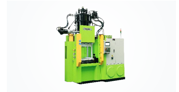
YL2-V200L带硅胶送料桶 (with silicone stuffer)
