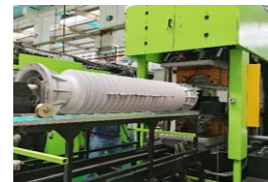
制品名称: 220kV管套 成型腔数: 一出二 Part Name: 220 kV Hollow Core Insulator Number of Cavities: 1
