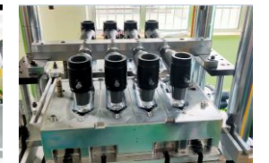
制品名称: 10kV T型接头 成型腔数: 一出八 Part Name: 10kV T Joint Number of Cavities: 8
