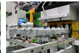
制品名称: 20kV复合横担 成型腔数: 一出四 Part Name: 20kV Composite Crossarm Number of Cavities: 4
