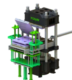
3 3RT双托 + 翻模 3RT double lifter + tilting device
