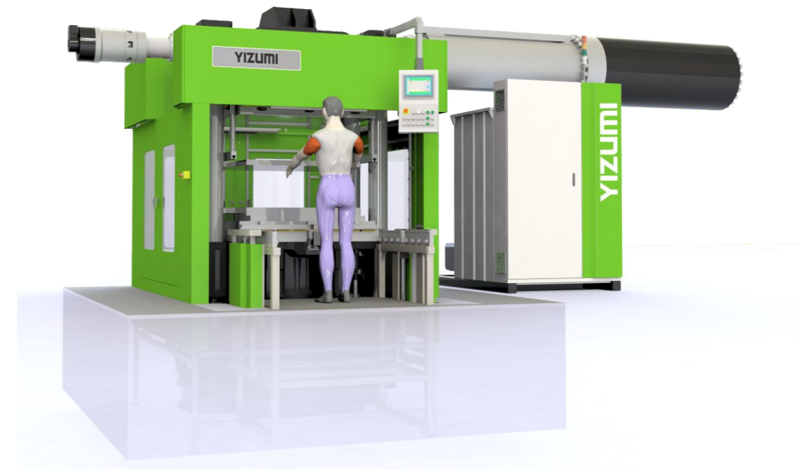
YL2-AB1200L (注射量40000cm 3 ,注射压力1900bar) (Injection volume 40000cm 3 , Injection pressure 1900bar)
