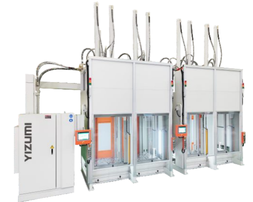
YL-V50 膜式空气弹簧硫化成型机 Rolling lobe air spring molding machine
